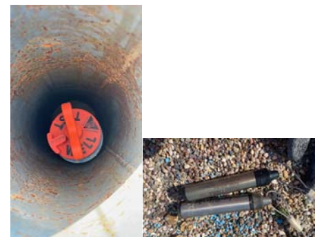
BH RC11. Upstand 0.39 m, two divers installed.
