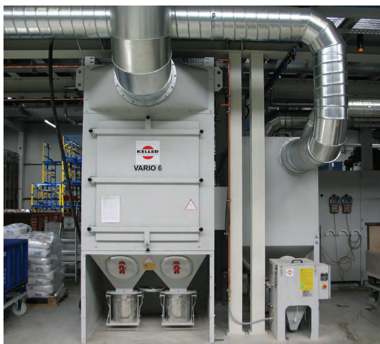
VARIO 6 with chip preseparation
