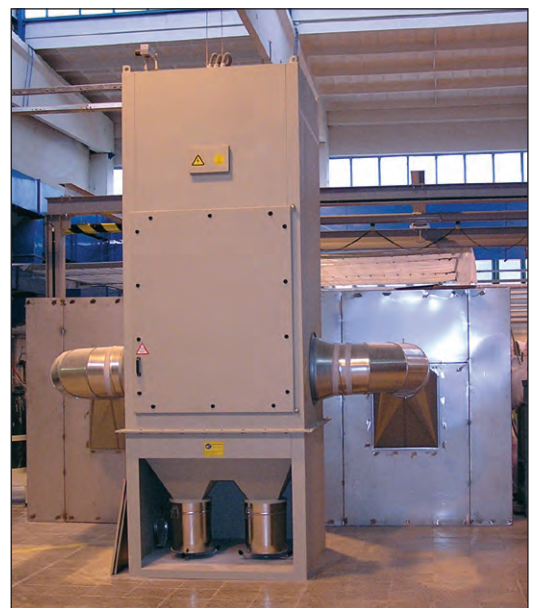
VARIO 3 for grinding cabin extraction
