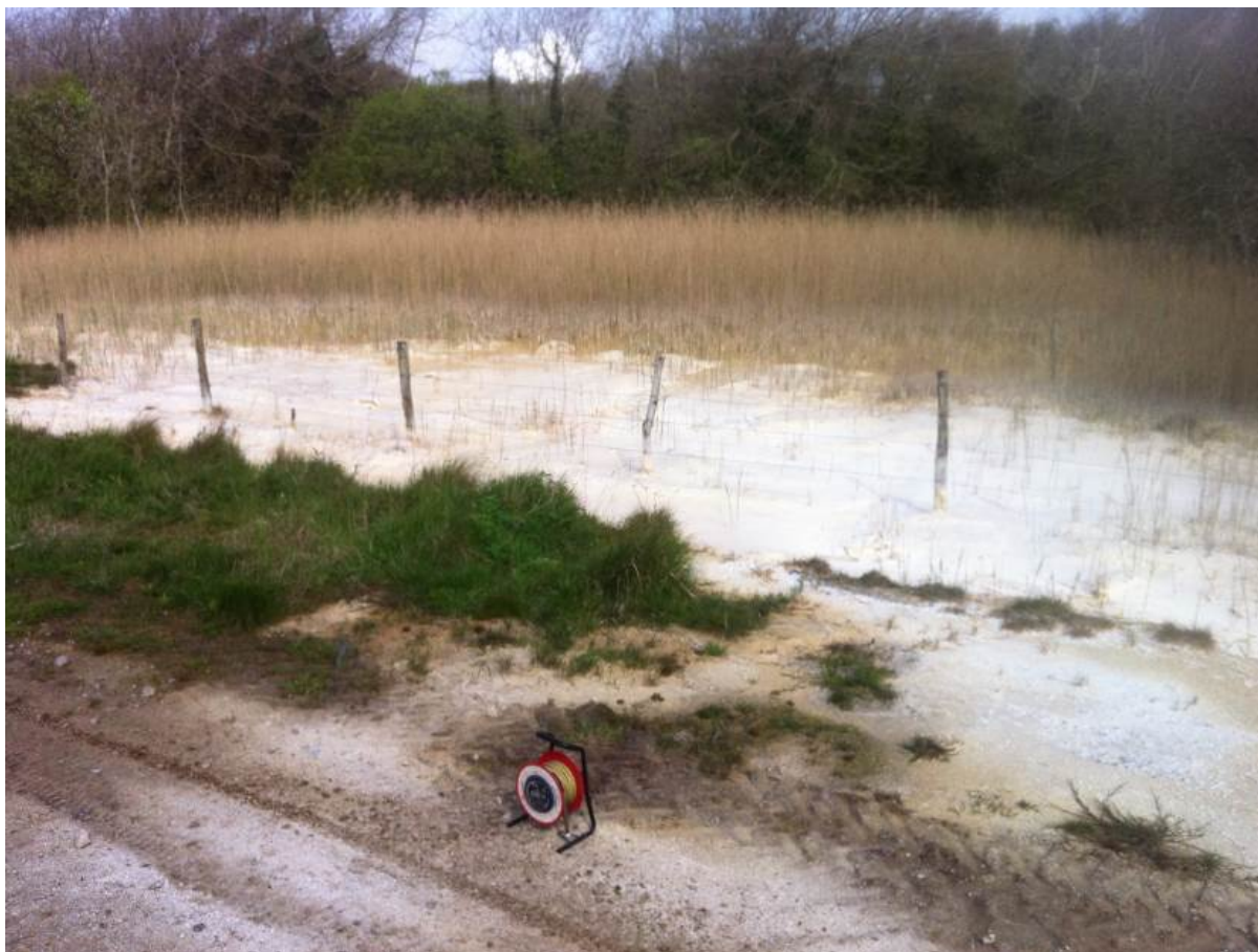
Plate 6-4 Accumulation of secondary precipitates adjacent to MCL (between BH17 and P12)
