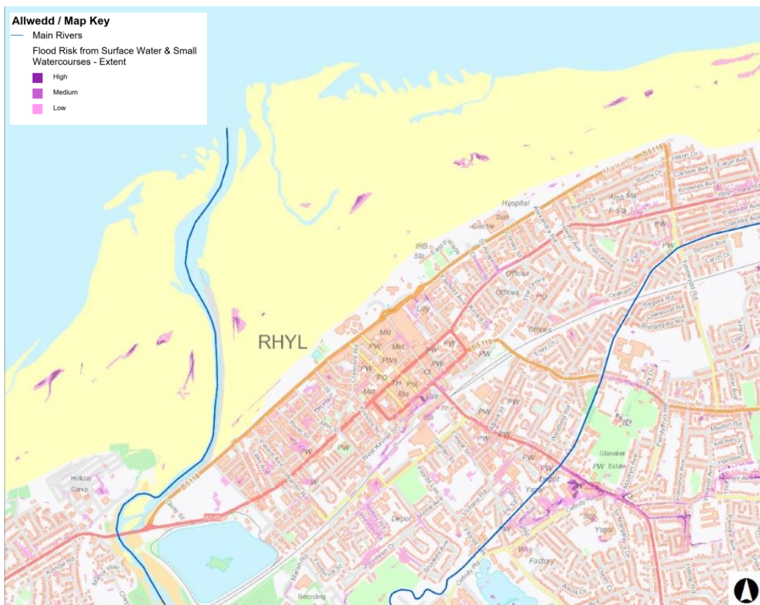
Figure 11.4: Central Rhyl Surface Water Flood Risk
