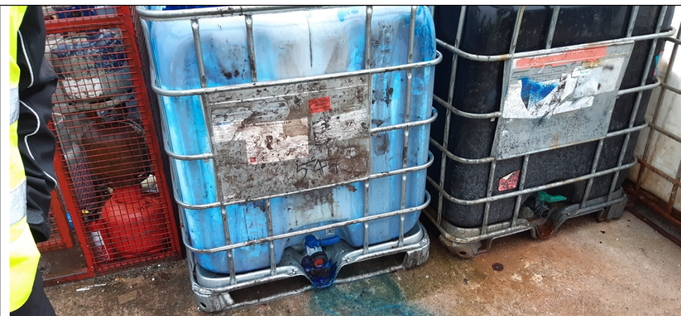
Photo 5 - IBC with blue liquid leaking from tap point
