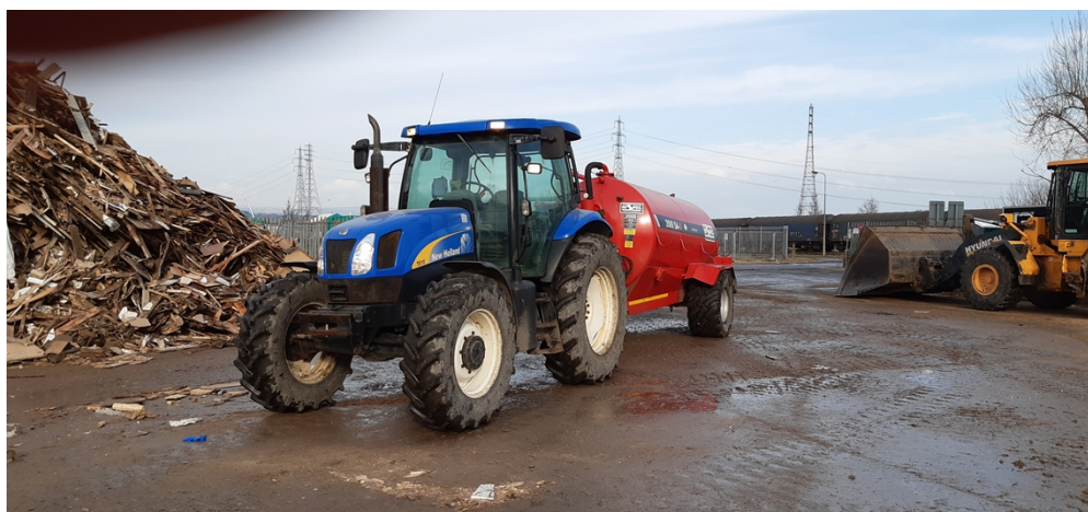
Photo 2 - Dust suppression system (tractor with water bowser) undertaking regular routine activities
