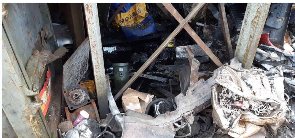
Photo 2 - Collection of oil and poor housekeeping near ELV depollution bay
