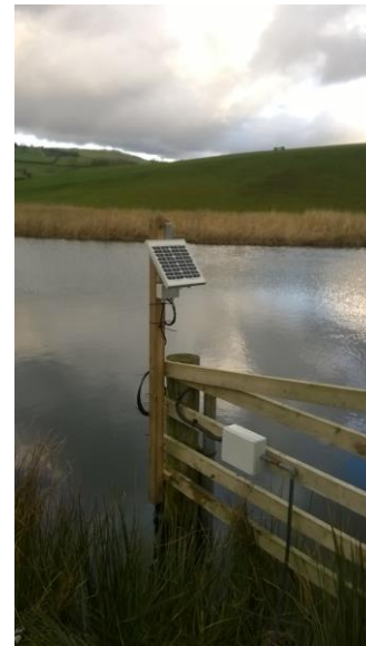
Figure 2: Example of a solar powered head level sensors with data logger and real time telecoms systems
