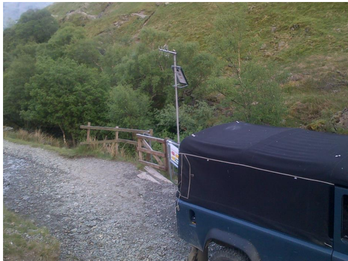
Figure 2: Example of a solar powered head level sensors with data logger and real time telecoms systems
