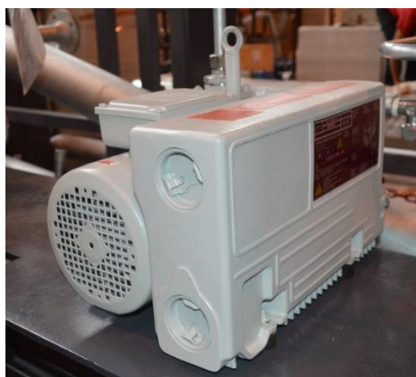
Figure 15.11-1: Vacuum pump.
