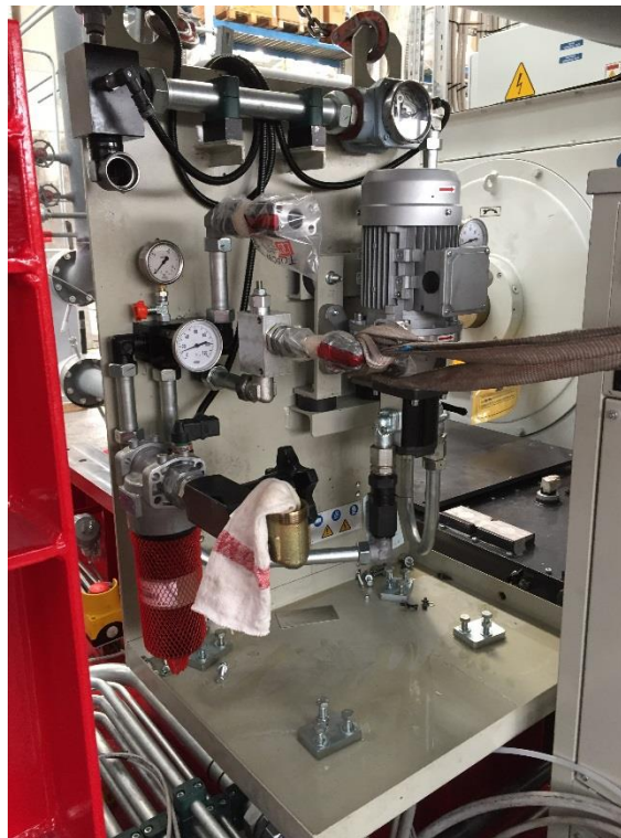
Figura 15.6-2: Pannel for lubrcated gearbox.
