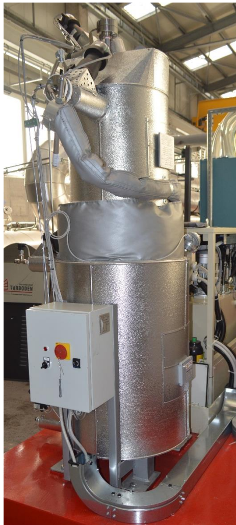
Figure 9.4-7: Oil separation system.
