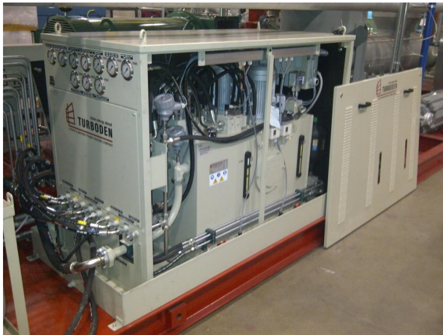
Figure 9.4-1: Lubrication control unit.
