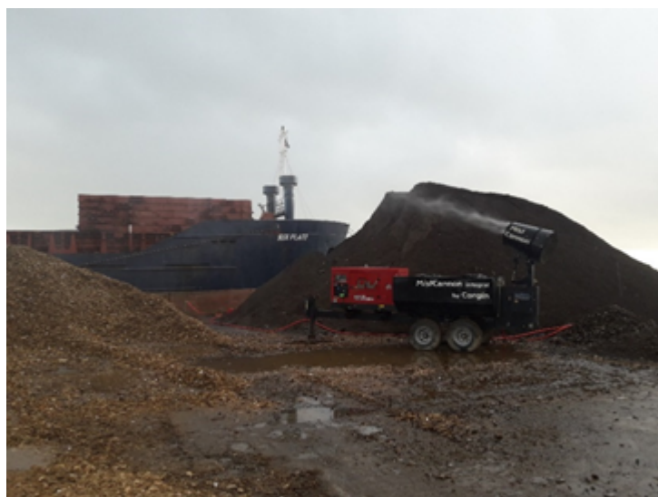
Figure 2 – use of mist cannon viewed during inspection on 15/12/2020
