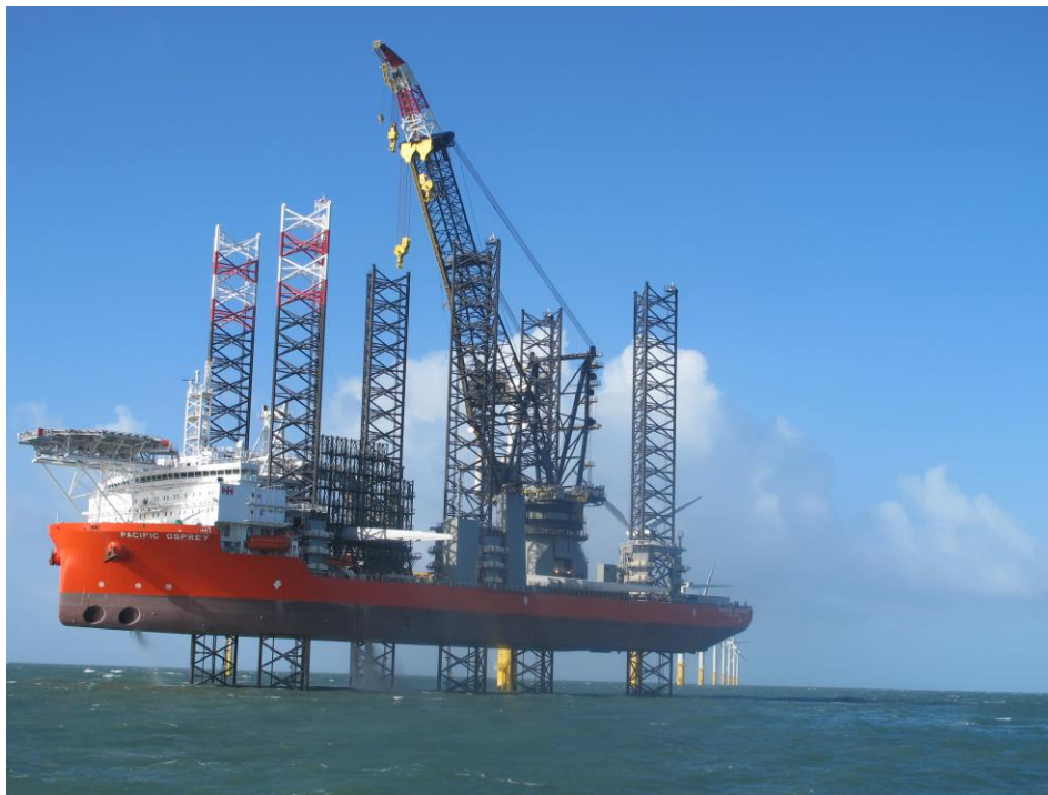
JUB in position for lifting operations
