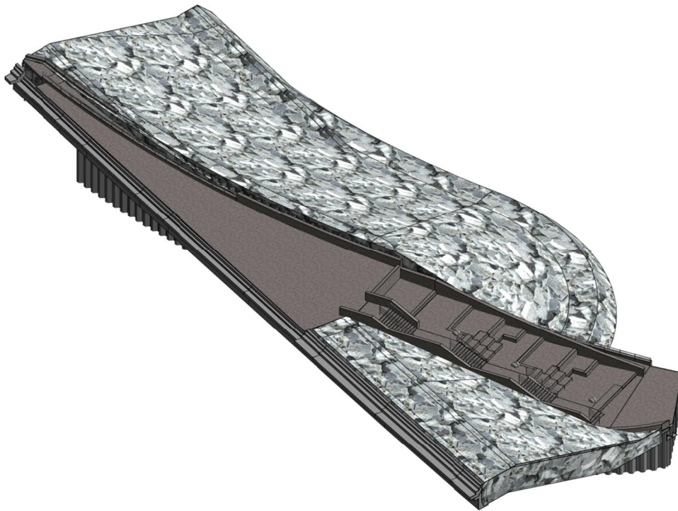
Figure 2.4: Perpendicular Access Steps 3D View
