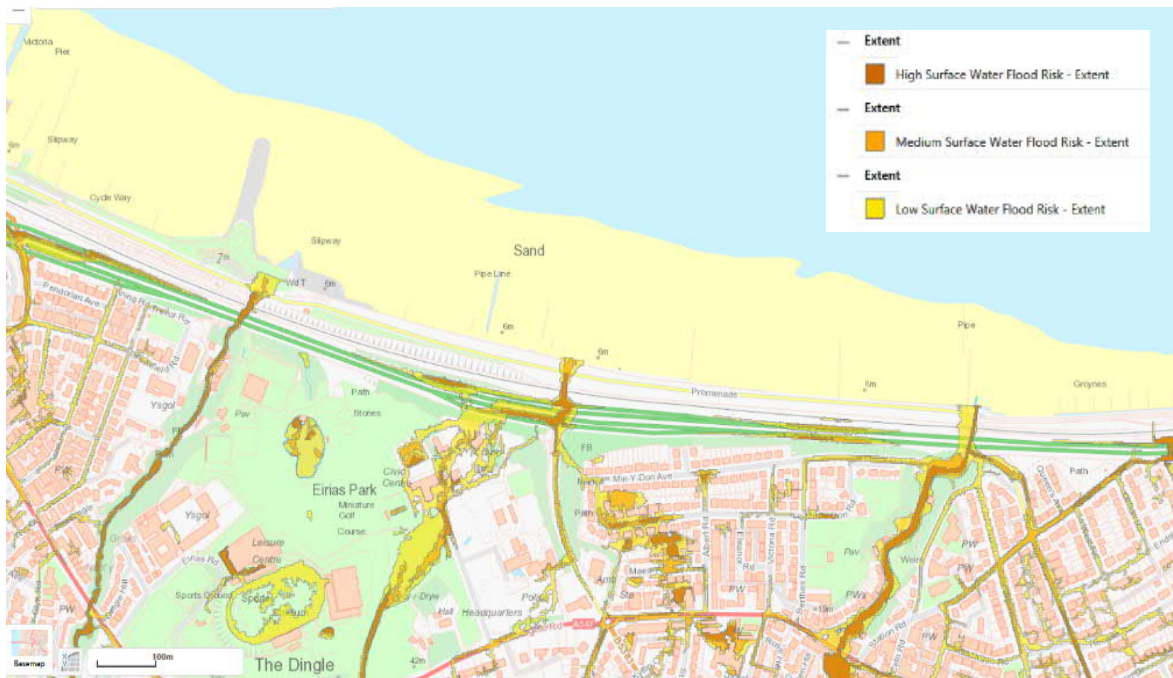
Figure 2.1: Colwyn Bay Surface Water Flood Risk
