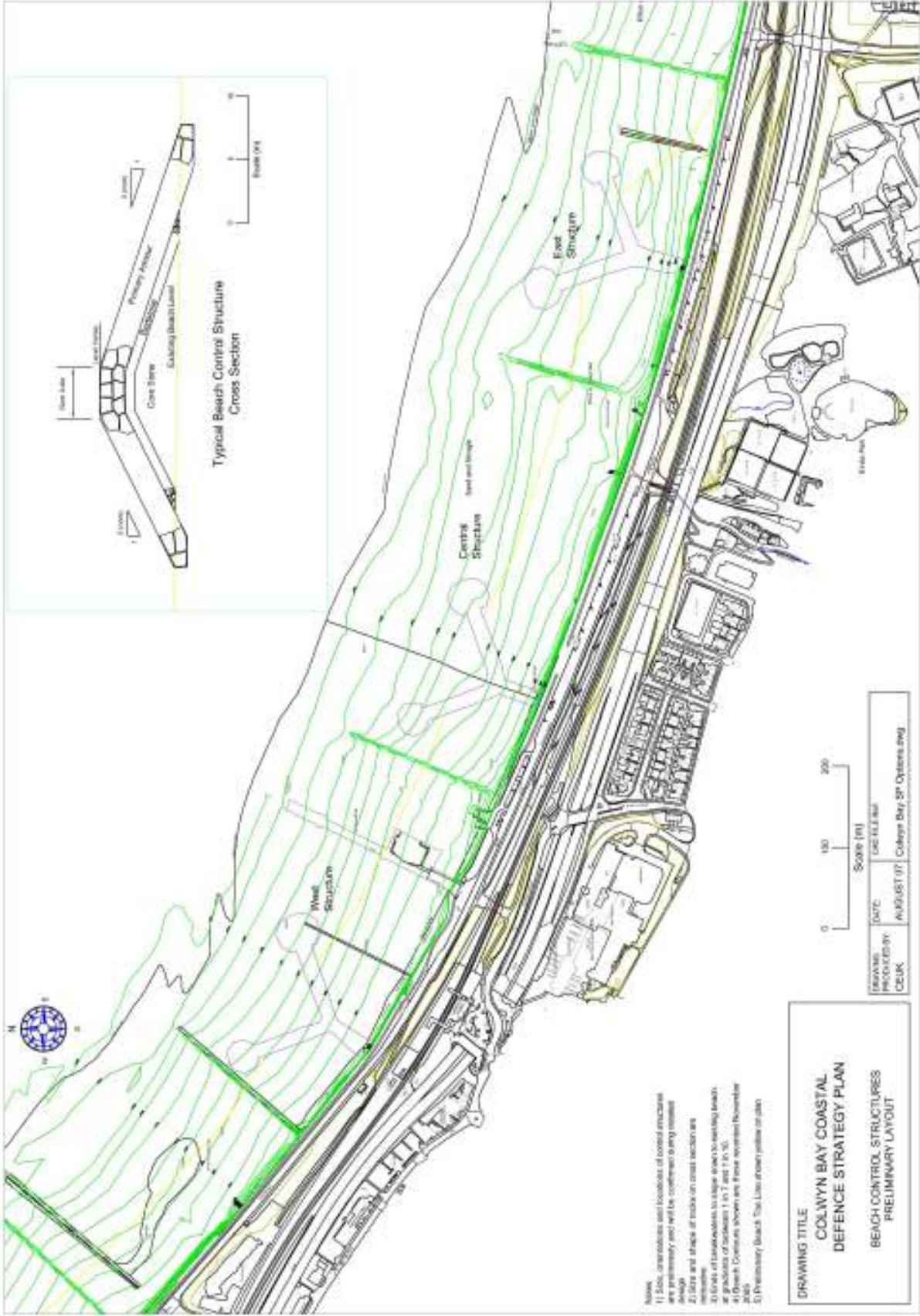
Figure 4.2 – Central Section: Preliminary Plan and Control Structure Cross Section
