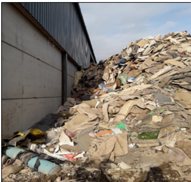
Image 11 – showing carpet waste pile stored up against the SRF unit with no clear gap
