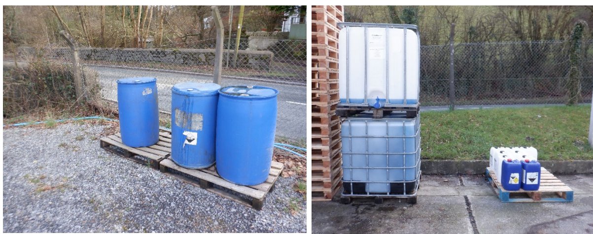
Figure 1 and 2 Showing potentially pollution liquids being stored without secondary containment
