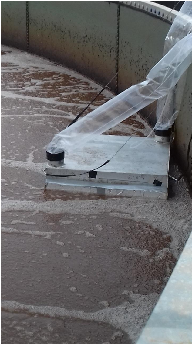
Figure 1 Odour Sampling with Lindvall Hood on the aeration tank.
