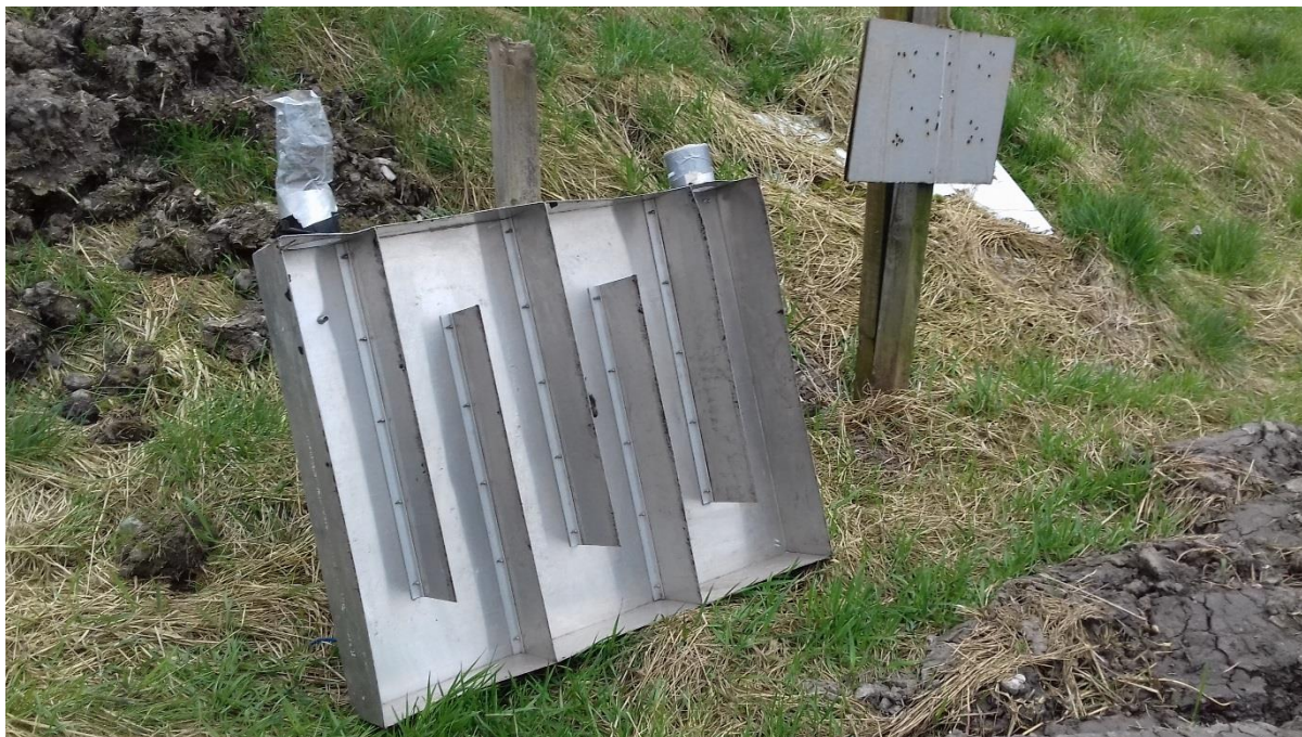
Figure 2 Underside of a Lindvall Hood showing the internal “vanes”
