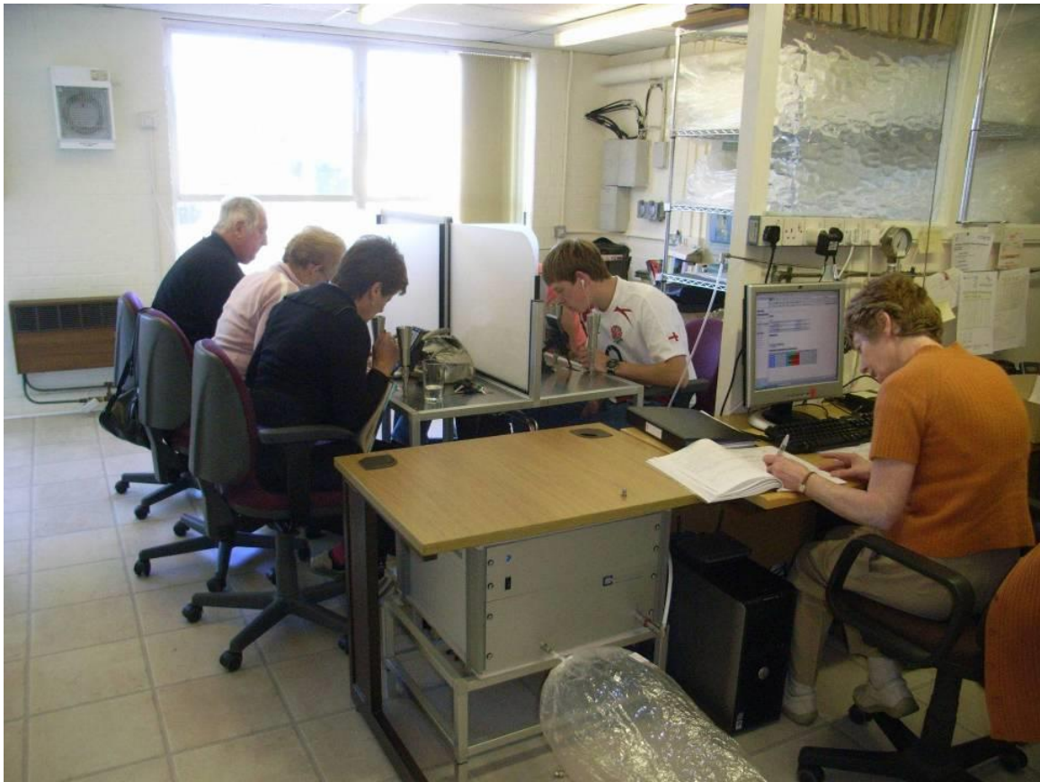
Figure 3 – Odour Analysis (sample bag in foreground)
