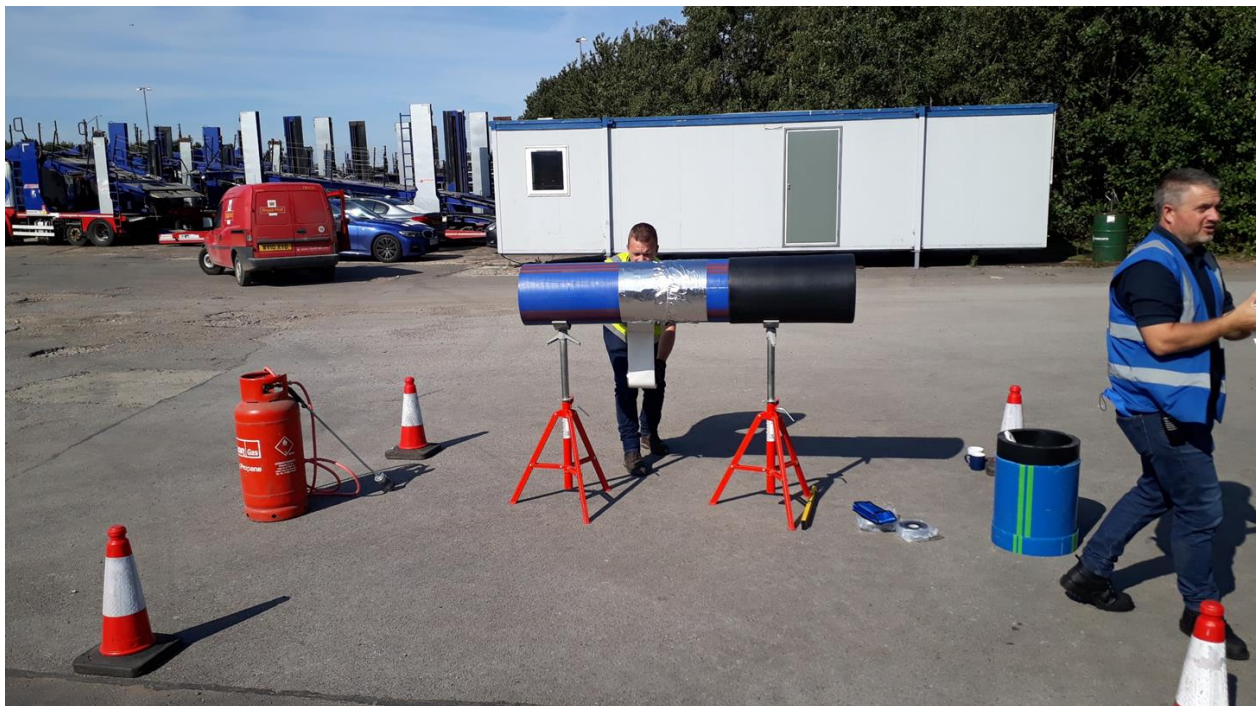
Diagram 21 : Pipeline Fabrication Stage 2 – Aluminium Wrapping
