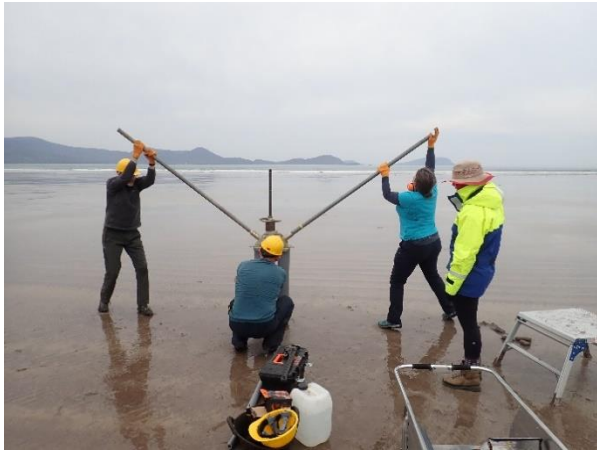
Figure 5. Core retrieval using the manual jacking system in the intertidal zone
