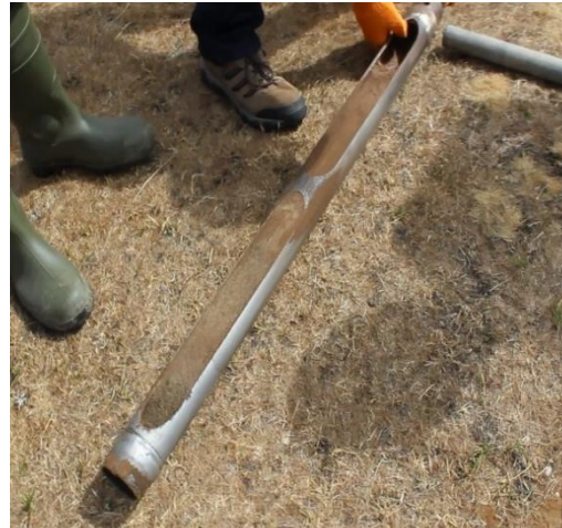
Figure 6 Impact of coring and example of extracted material in an open barrel corer
