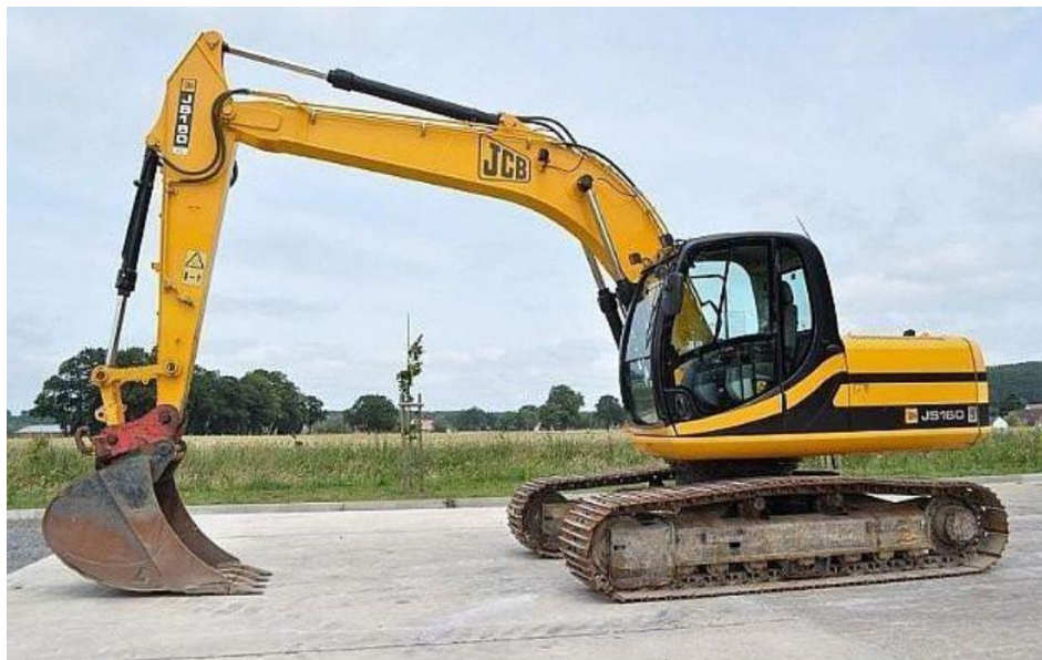
Figure 1-2 - Tracked Excavator with Bucket for Excavation
