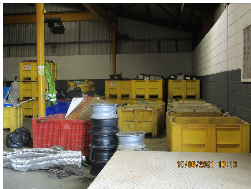
Figure 3. Batteries stored in acid resistant containers which are situated inside the warehouse.
