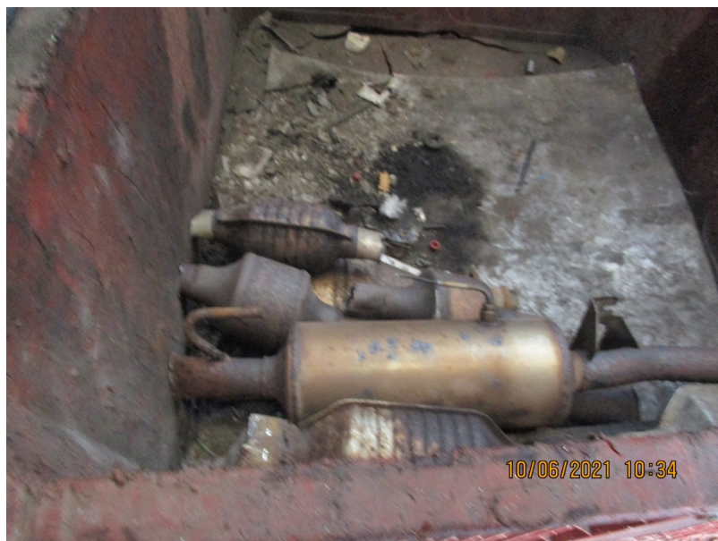
Figure 4. Catalytic converters in acid resistant containers which are situated inside.
