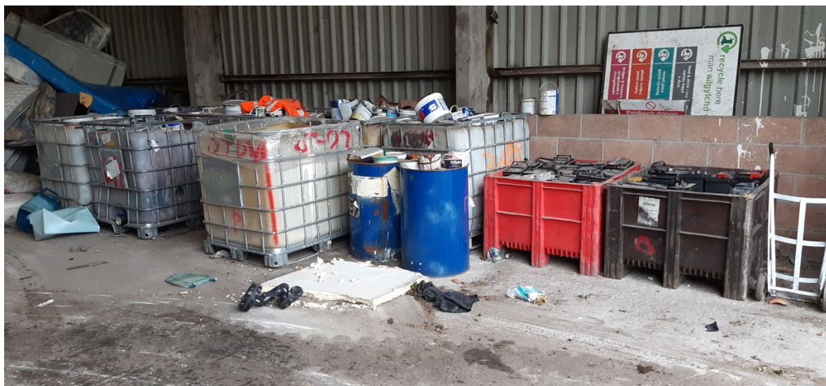
Photo 3 - Hazardous waste storage within interceptor drainage system area
