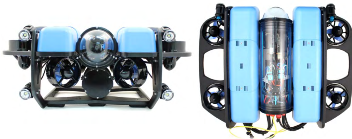
Plate 3 OEL's BlueROV II Remotely Operated Vehicle (ROV) used for inspection of Holyhead Breakwater bullnose.
