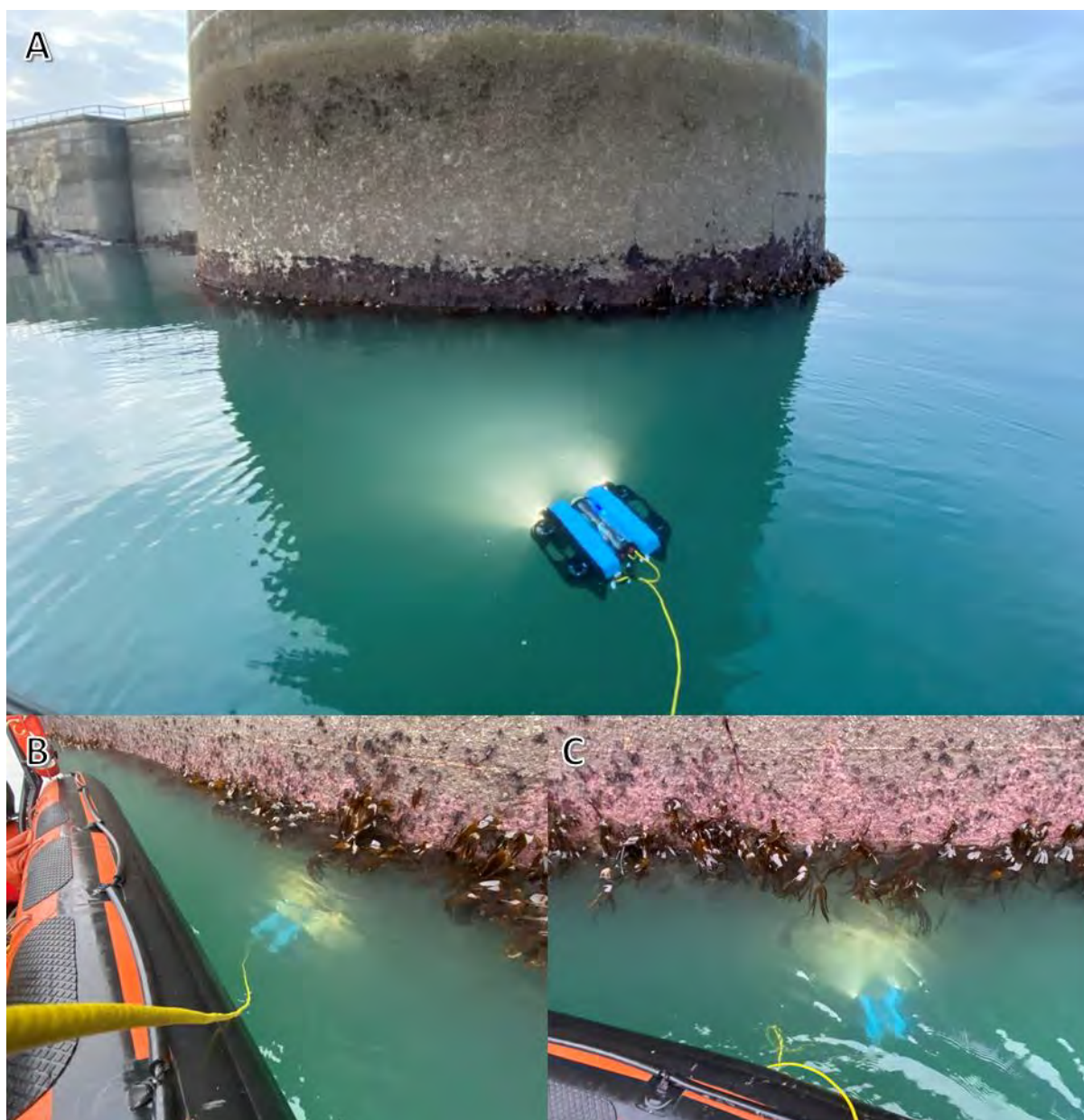
Plate 4 OEL's BlueROV II ROV sampling the Holyhead Breakwater bullnose A) BlueROV II approaching bullnose from the south B & C) BlueROV II inspecting bullnose wall below waterline.
