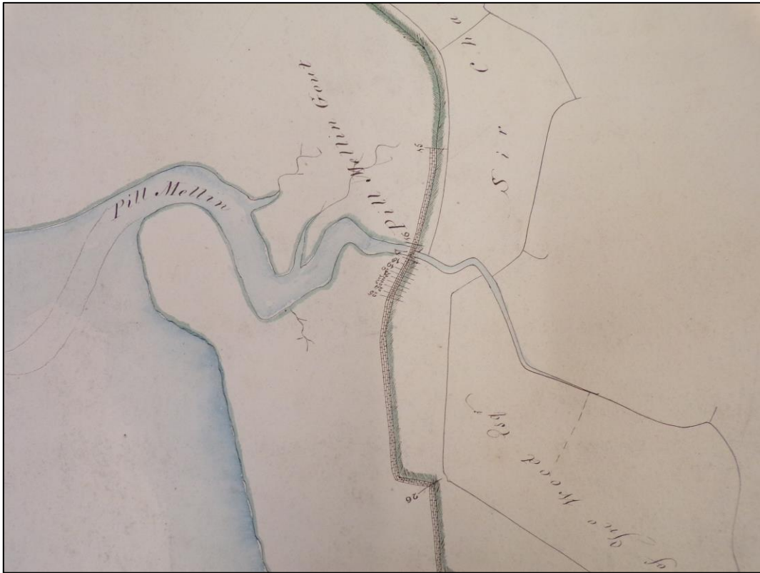
Plate 3: Detail from the 1823 survey of the sea walls in the manor of Rumney. Note that the defences at the bottom of the map (approximately southeast) are shown to be a bank revetted with stone. To the north, it is largely an earthen bank.
