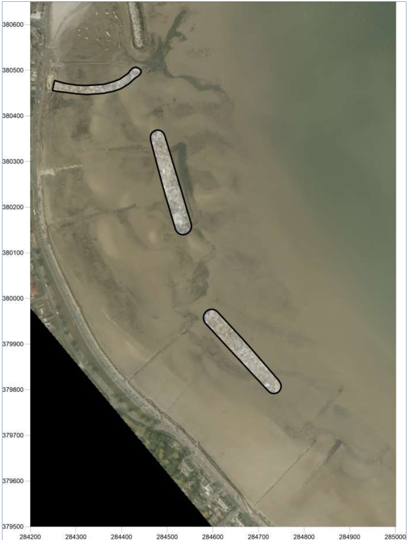
Figure 7: Option 4b: Proposed Control Structure Layout
