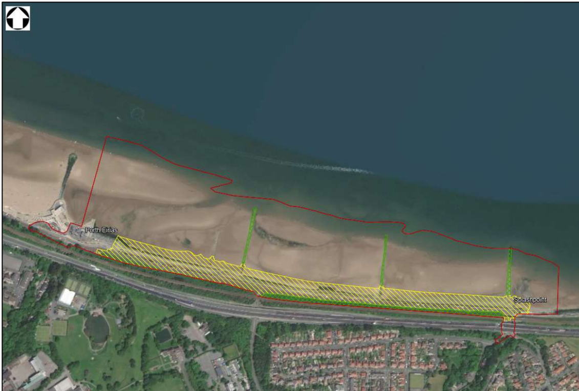
Figure 1.4: Old Colwyn Coastal Defence and Active Travel Scheme red line boundary and areas of permanent construction (yellow hatching, green hatching relates to ecological mitigation areas)
