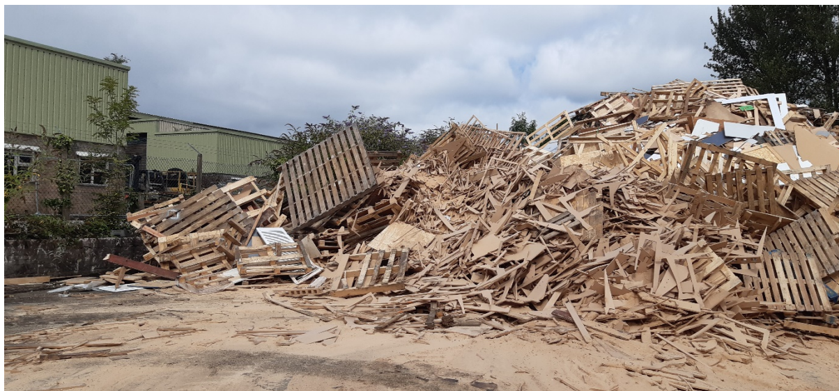
Image 4 – showing new location for wood waste, limited separation distance between waste and site boundary.
