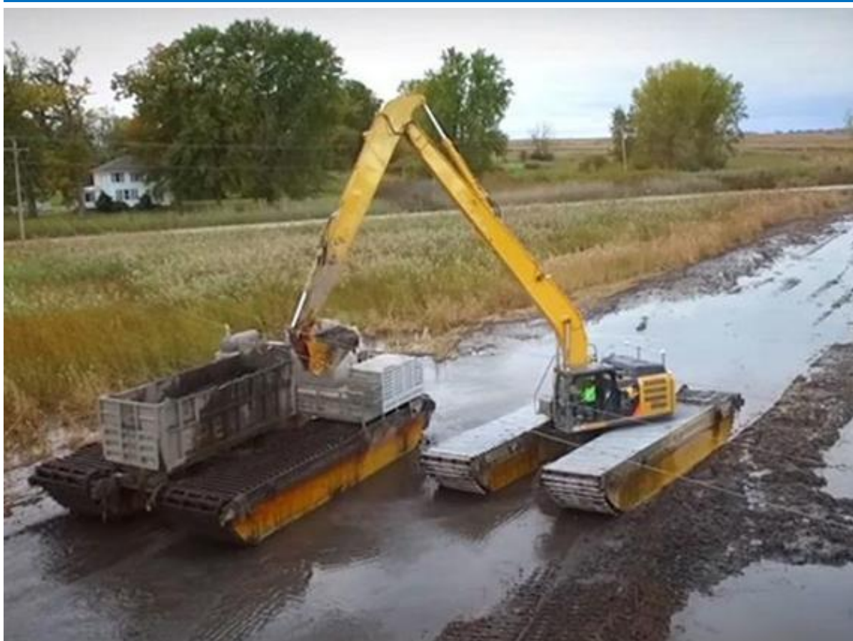
Figure 3-3: An amphibious excavator will be used to unload and place the turf without damaging it.
