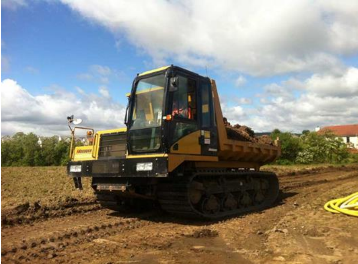
Figure 3-2: Harvested turf will be loaded onto flat backed ultra low ground pressure tracked dumpers
