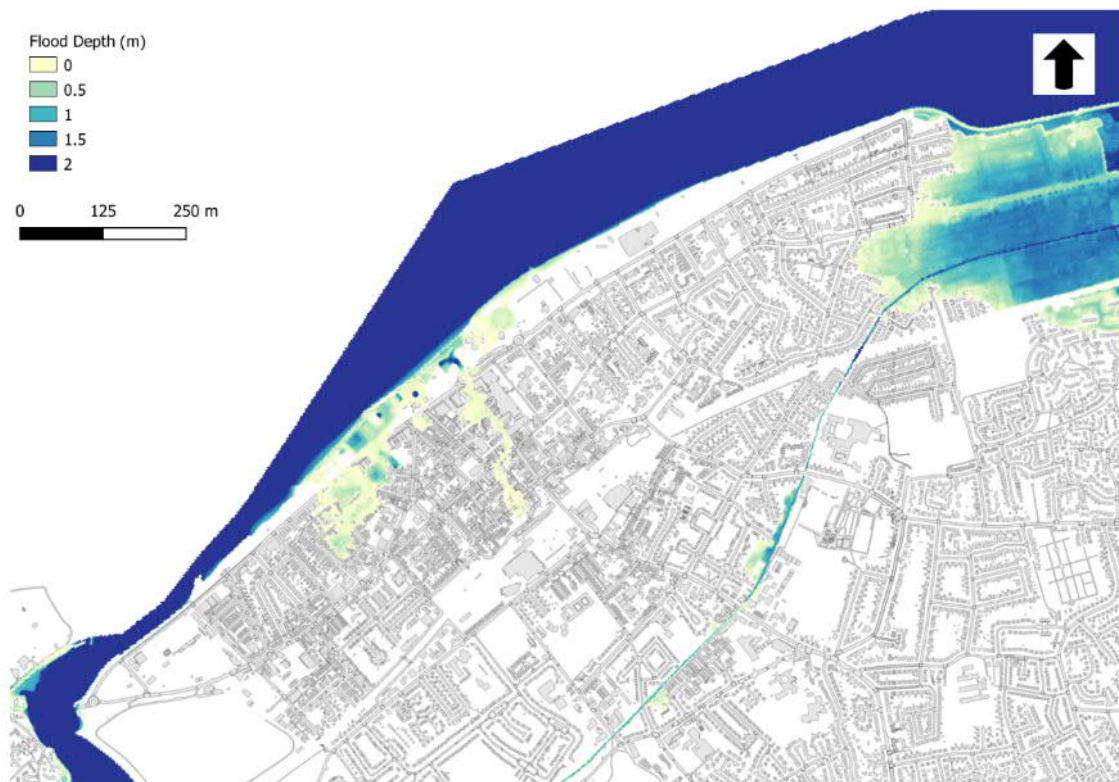
Figure 5.4: Section E-H Only – 15l/s/m Overtopping Rate
