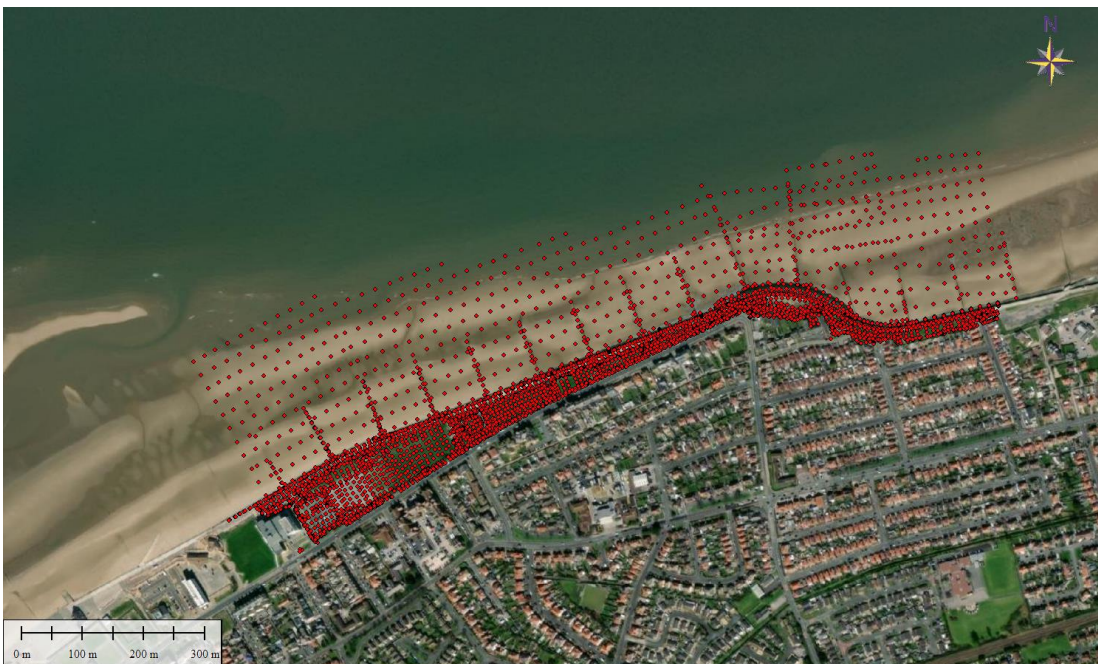
Figure 2.10: Location of topographic data points in a post-storm beach survey in December 2013.
