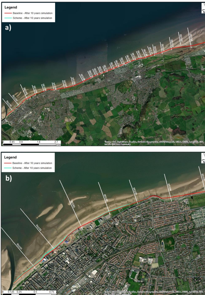
Figure 5.25: Position of the baseline coastline (red line) and the Scheme coastline (light blue line) after the ten-year coastline evolution simulation for: a) the entire study area, from Rhyl to the Point of Ayr; and b) Central Rhyl to Splash Point.
