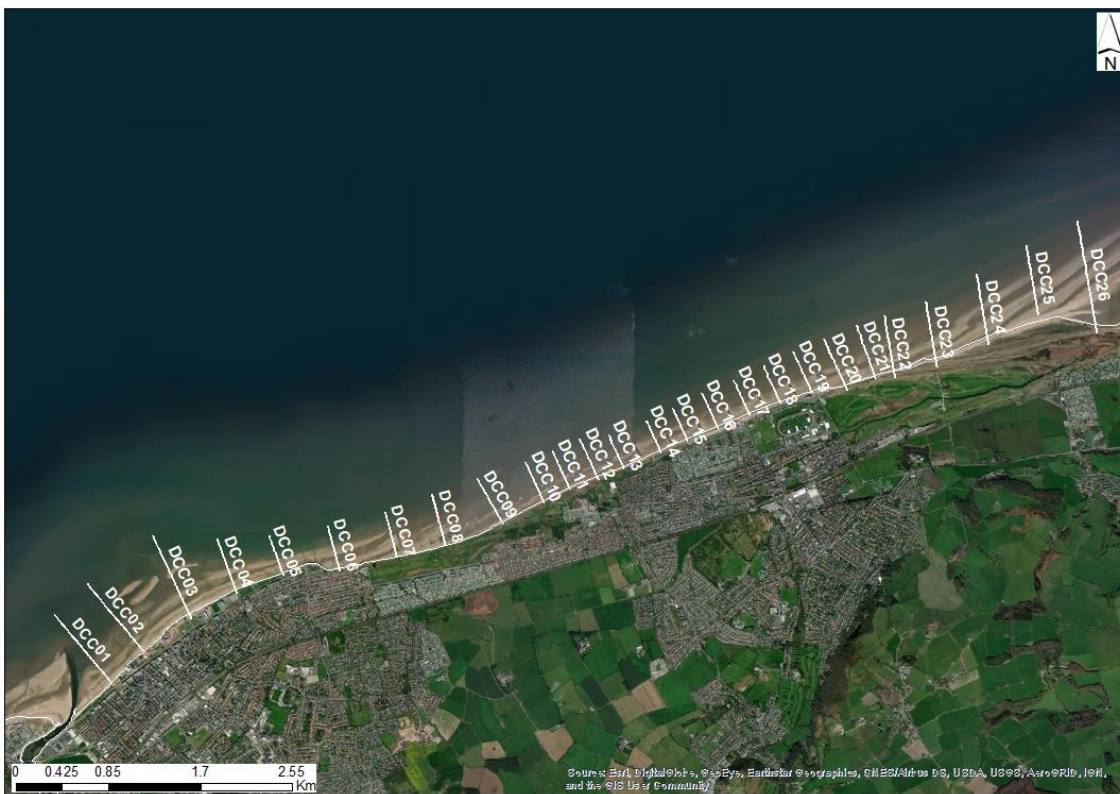
Figure 5.2: Cross-shore profiles selected to represent the North Wales coastline, between the River Clwyd and the Point of Ayr.
