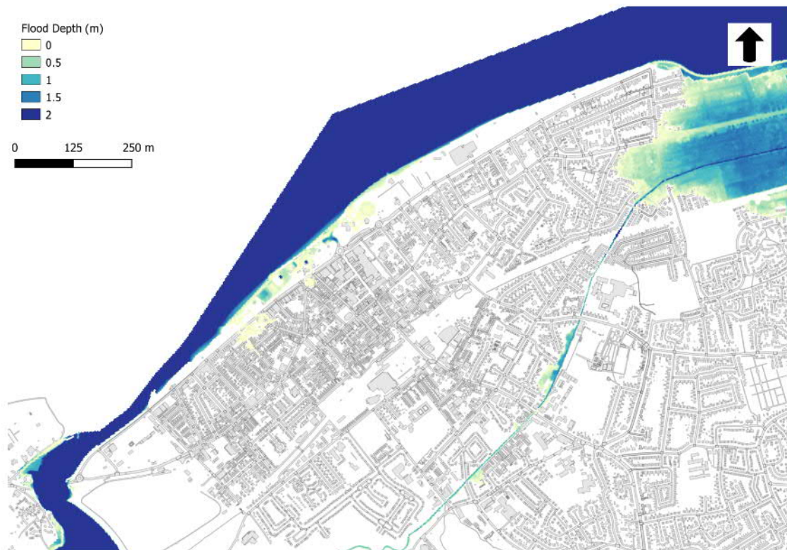
Figure 5.6: Section E-H Only – 5l/s/m Overtopping Rate
