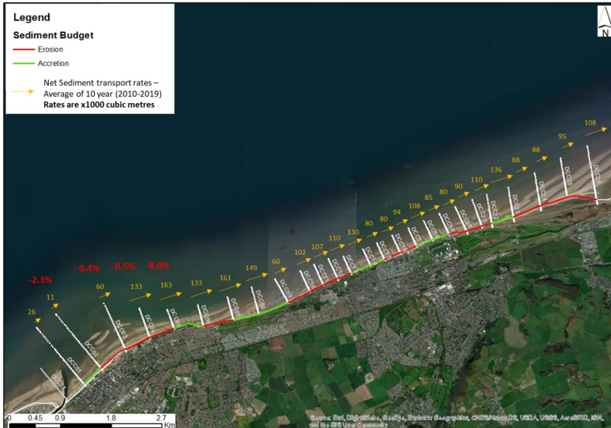
Figure 5.9: Simulated yearly net longshore sediment transport rates ( Q_{LST} ) values for each cross-shore profile, including the proposed Scheme between profile DCC01 and DCC05. A positive transport rate indicates transport from west to east. The green and red coastline lines show the estimated sediment budget. A negative budget indicates erosion between the two profiles. Compared to the baseline case, the change in the transport rates is shown as percentages in red.
