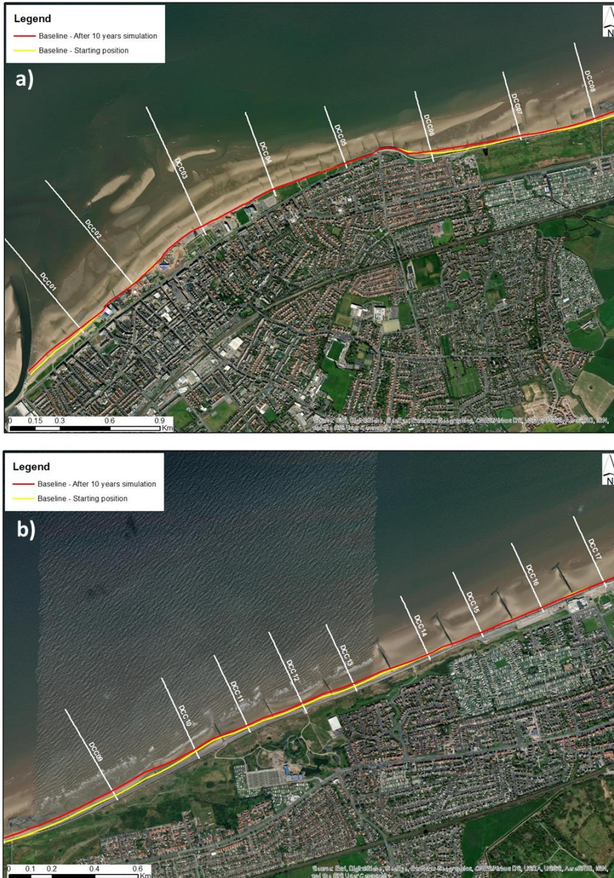
Figure 5.22: Position of the coastline at the start (yellow line) and at the end (red line) of the ten year coastline evolution simulation for two specific areas. a) Central Rhyll and a portion of East Rhyll; b) frontage between East Rhyll and Prestatyn.
