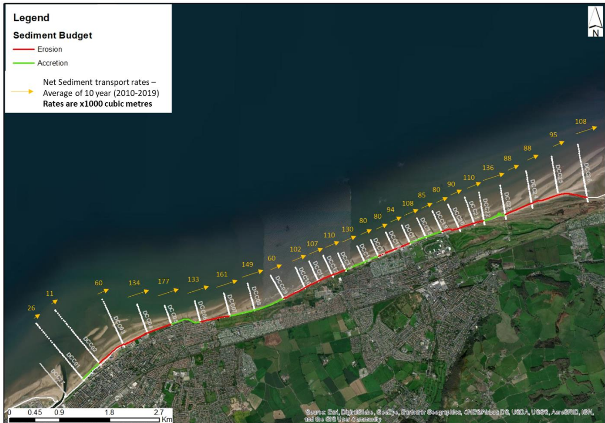
Figure 5.6: Simulated yearly net longshore sediment transport rates ( Q_{LST} ) for each cross-shore profile. A positive transport rate indicates transport from west to east. The green and red lines show the estimated sediment budget. A negative budget indicates erosion between the two profiles.
