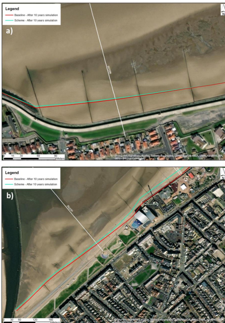
Figure 5.26: Enlarged view of the position of the baseline coastline (red line) and the Scheme coastline (light blue line) after the 10-year coastline evolution simulation for: a) beach section after Splash Point; and b) the beach section behind the training wall at Central Rhyl.
