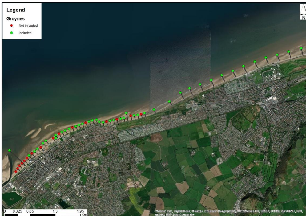
Figure 5.19: Location of all groyne structures, including training wall, wooden, concrete and fish tail groynes, on the coastline between Rhyl and the Point of Ayr. The groynes shown in red are excluded from the baseline model simulation.
