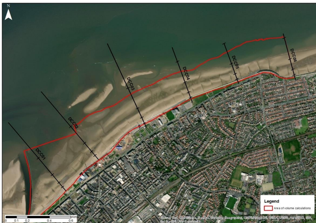
Figure 3.10: Area (red box) used for the volume change calculation between LiDAR surveys.
