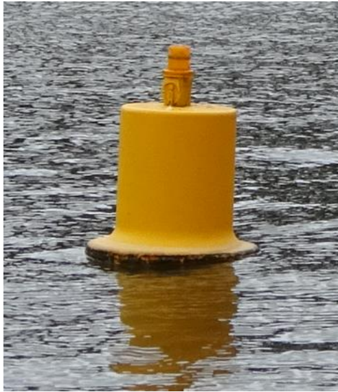
Figure 6. The proposed farm will be clearly marked by six yellow special mark Trinity House buoys (spherical or pillar). A yellow 'X' shaped top mark and lit at night by Fl.Y.5s yellow flashing lights.
