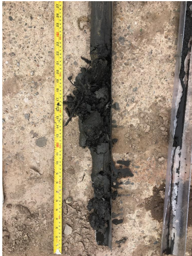
Photograph 6 - Photograph taken of the water saturated organic rich horizon identified at 4.60m within BH5
