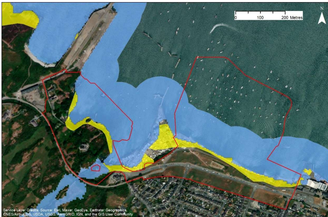
Figure 3-3: TAN15 Development Advice Map (WMS Layer) overlaid onto Google Aerial Imagery. Zone C2 = Blue, Zone B = Yellow, Zone A = Clear
