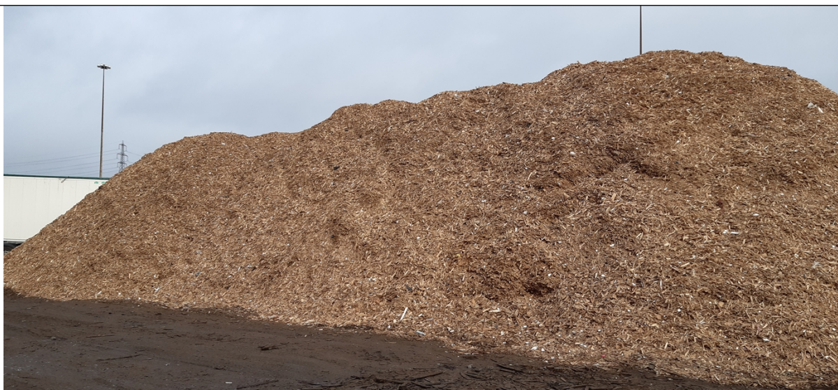
Photo 2 - Wood stockpile size within 4 metre recommended maximum height
