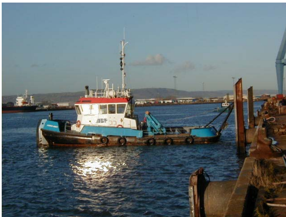
Plate 6. A plough vessel pulling material from the toe line of a berth face to a location where the TSHD can access it.
