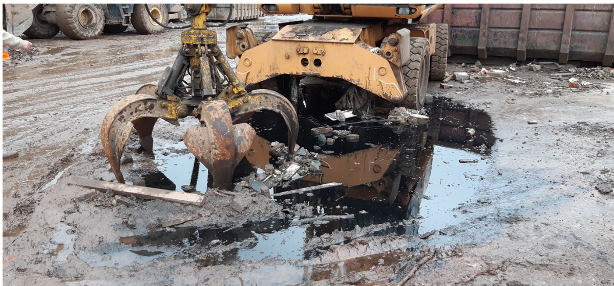
Photo 2 - Pool of excess oil originating from broken down plant
