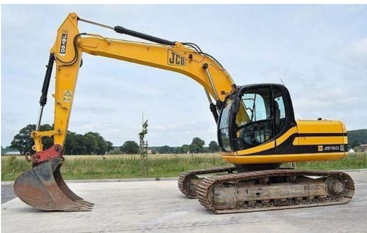
Figure 3-1 Tracked Excavator with Bucket for Excavation
