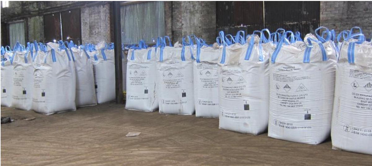
Photograph 3.3: Typical Storage arrangements of EAF dust within a warehouse
