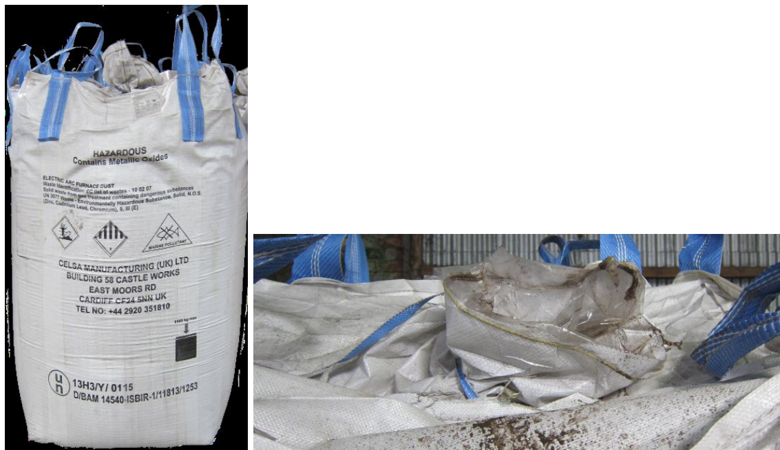
Photograph 3.1: EAF Big Bags (showing plastic liner)
