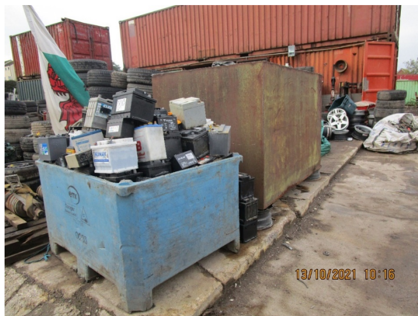
Figure 4. Waste batteries stored in an acid proof banded container without a cover and with some batteries stored on the floor without any container or cover.
