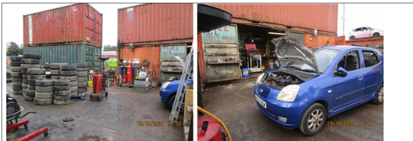
Figure 1. Depollution bay where ELV's are depolluted.
