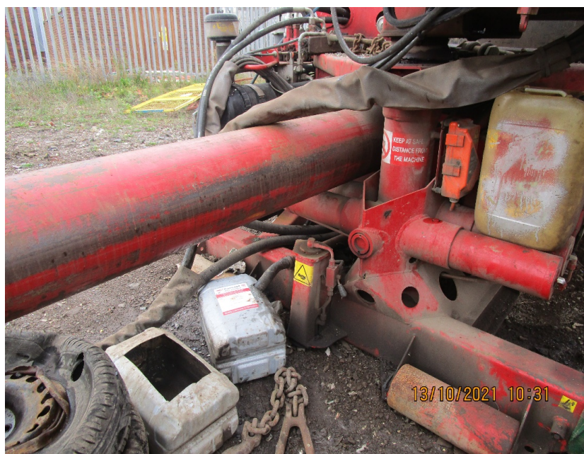
Figure 10. Container connected to external piping that collects waste oil produced from the crushing process.
