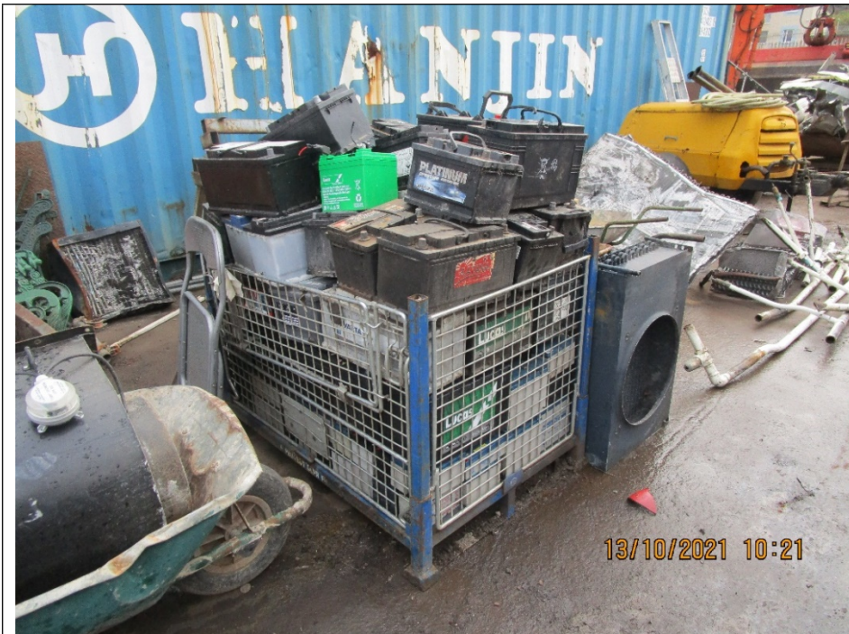
Figure 5. Waste batteries stored in an unsuitable container that is not acid-proof, not bunded nor has any cover.
