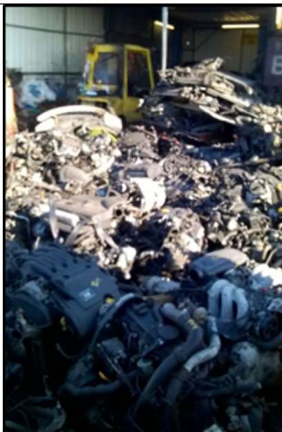
Picture 1 – showing depolluted engines stored on impermeable surface
