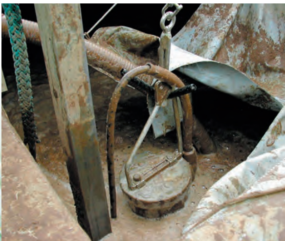
Submersible AirJet for agricultural waste
