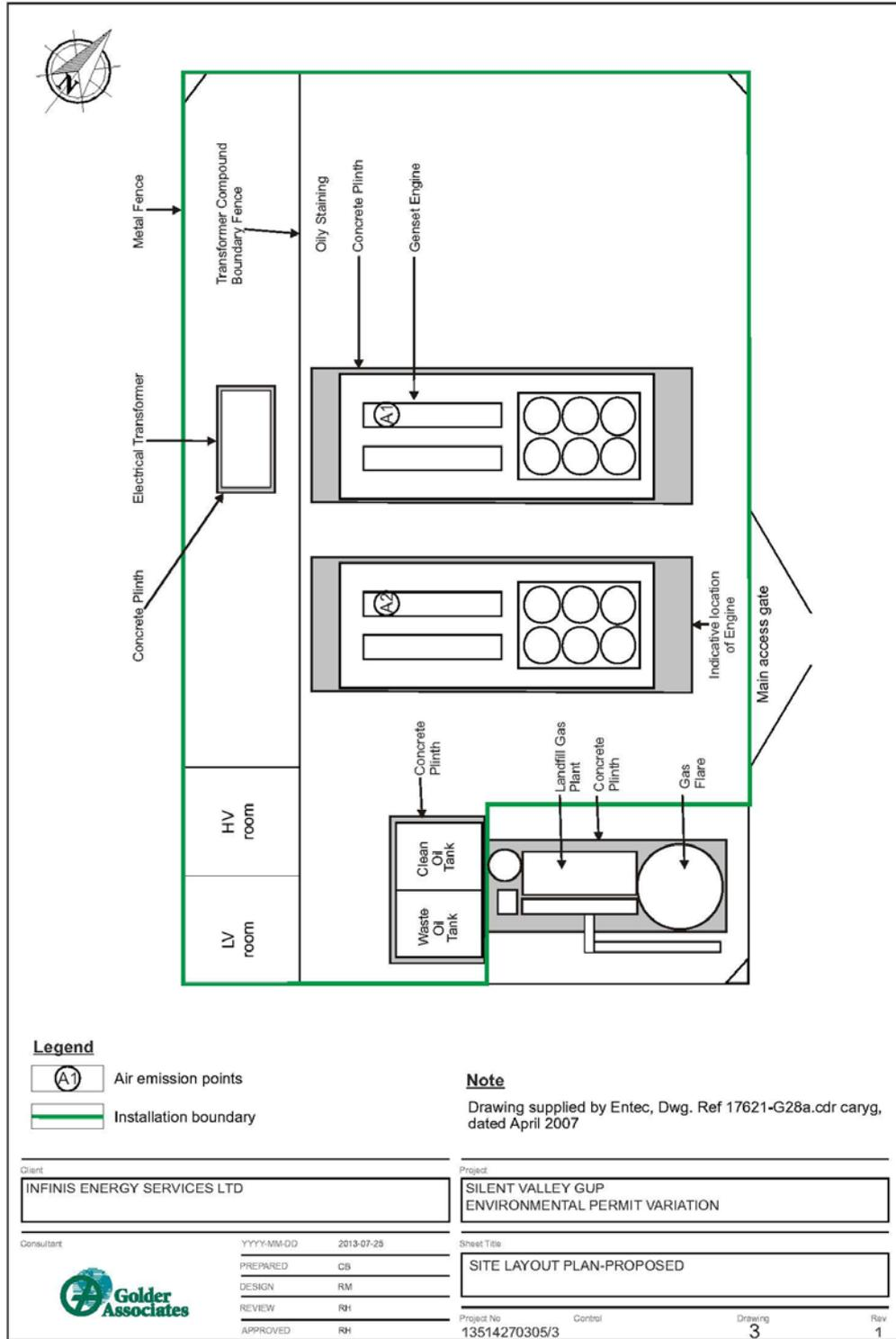
The plan above shows the layout of the gas engines in the Gas Utilisation Plant.
