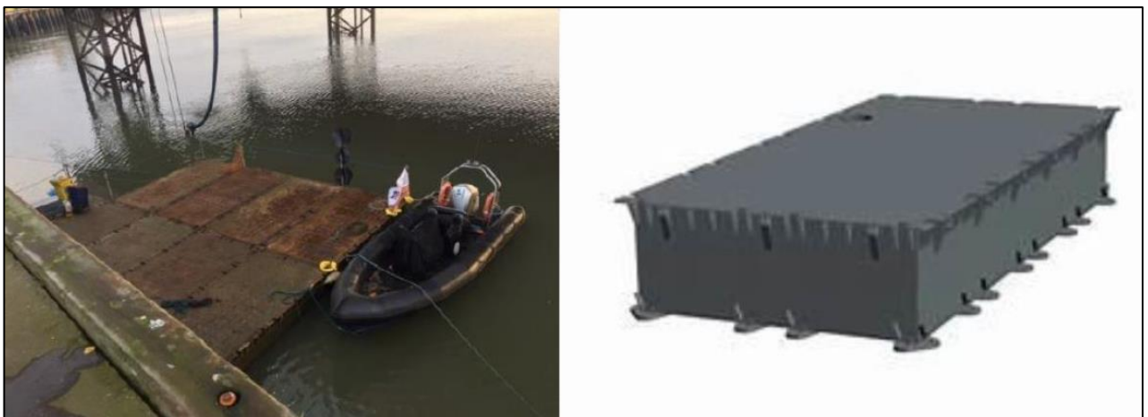
Figure 12: Example of metal pontoon platforms.
