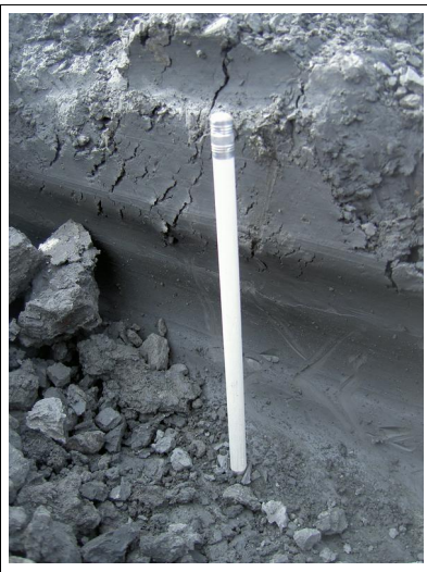
compacted clay horizon
