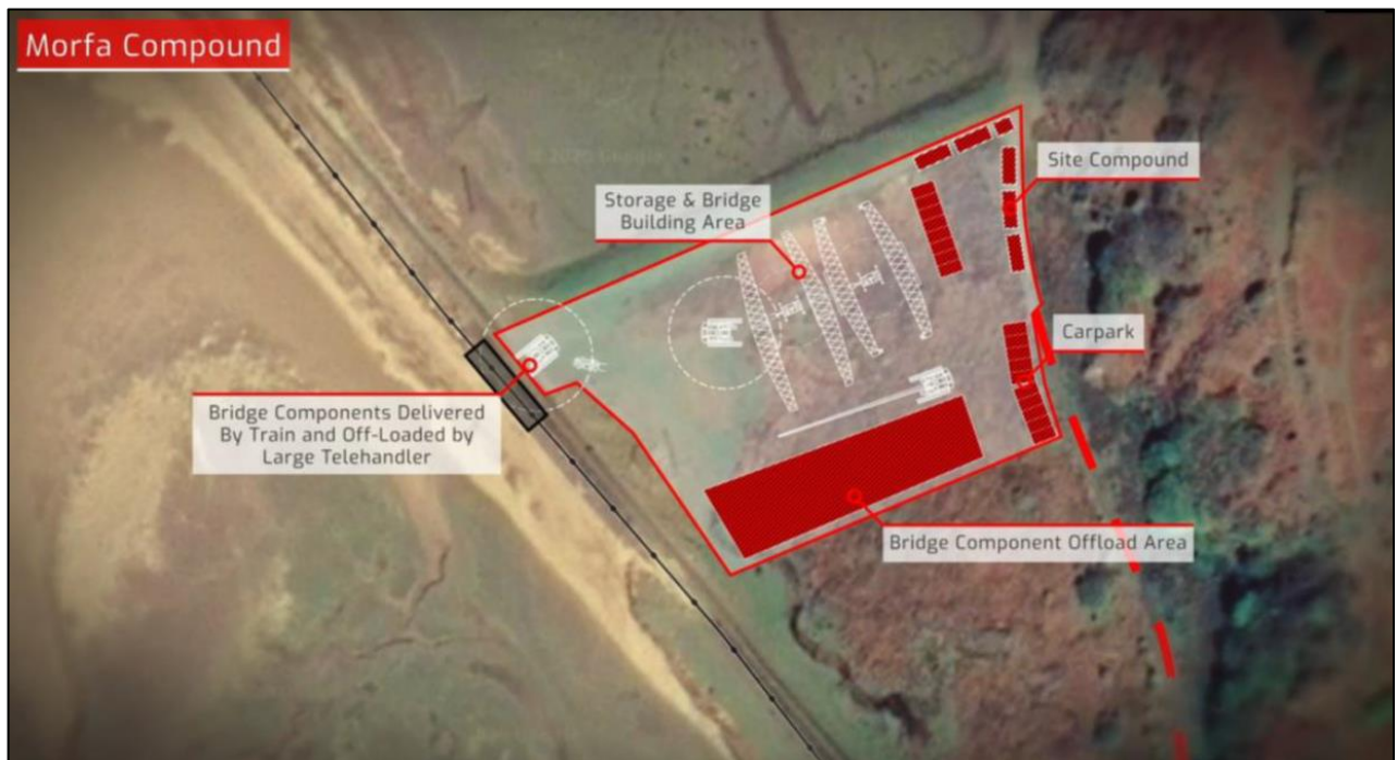
Figure 8: Upgraded compound to support new metallic sections.
