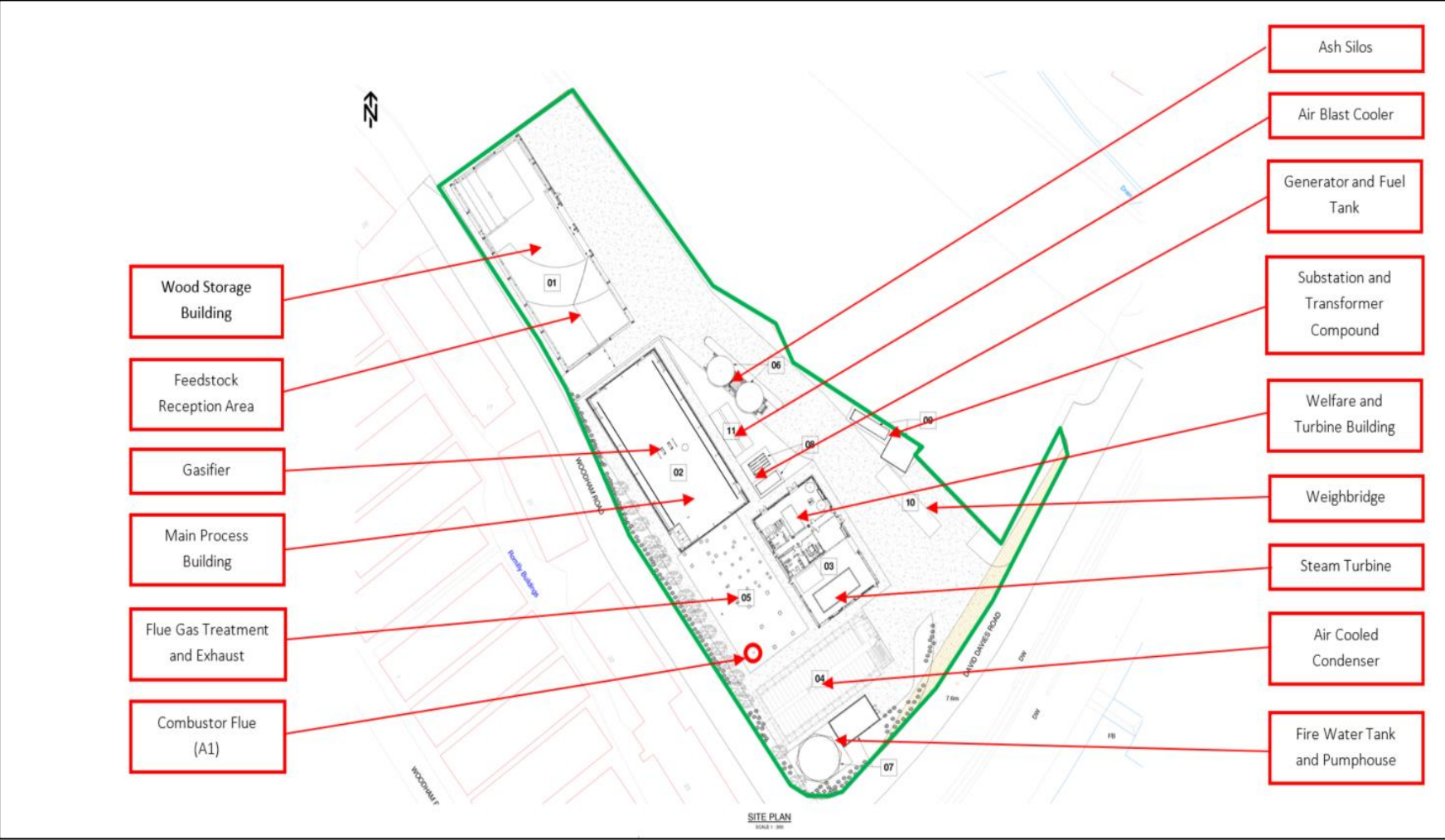
Figure 3: Major site plant, buildings and processes
