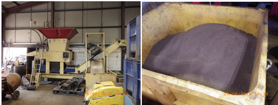
Granulation machine and waste plastic produced
