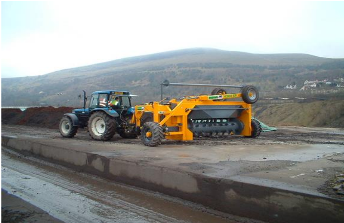
Figure 3-3 Bioremediation Process – Mechanical Turning (Menart)
