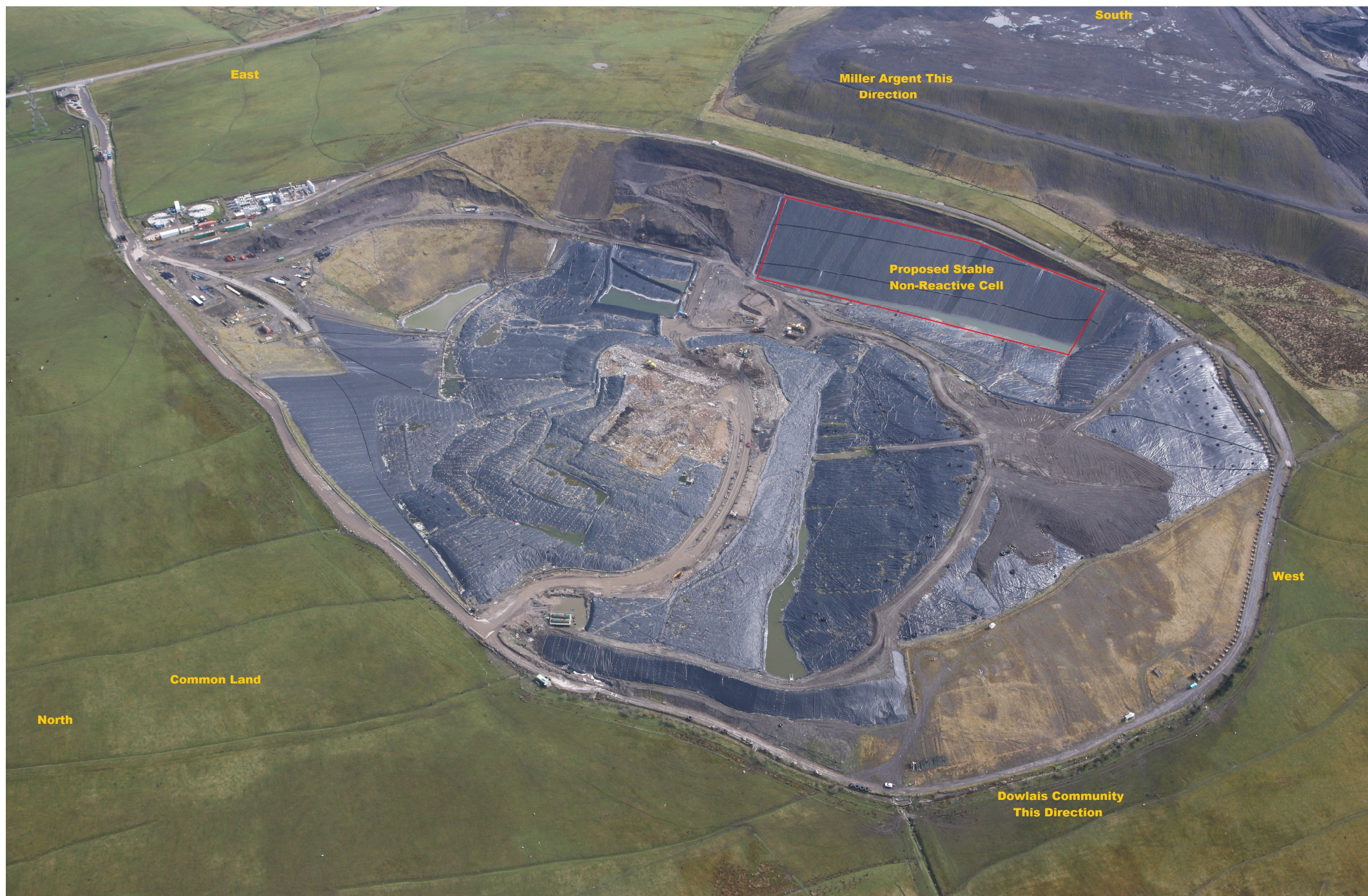
Figure 2. Aerial view of Trecatti Landfill Site showing the location of the stable non-reactive cell for asbestos. Please note that this image was used in the permit application, the asbestos cell has since been built.
