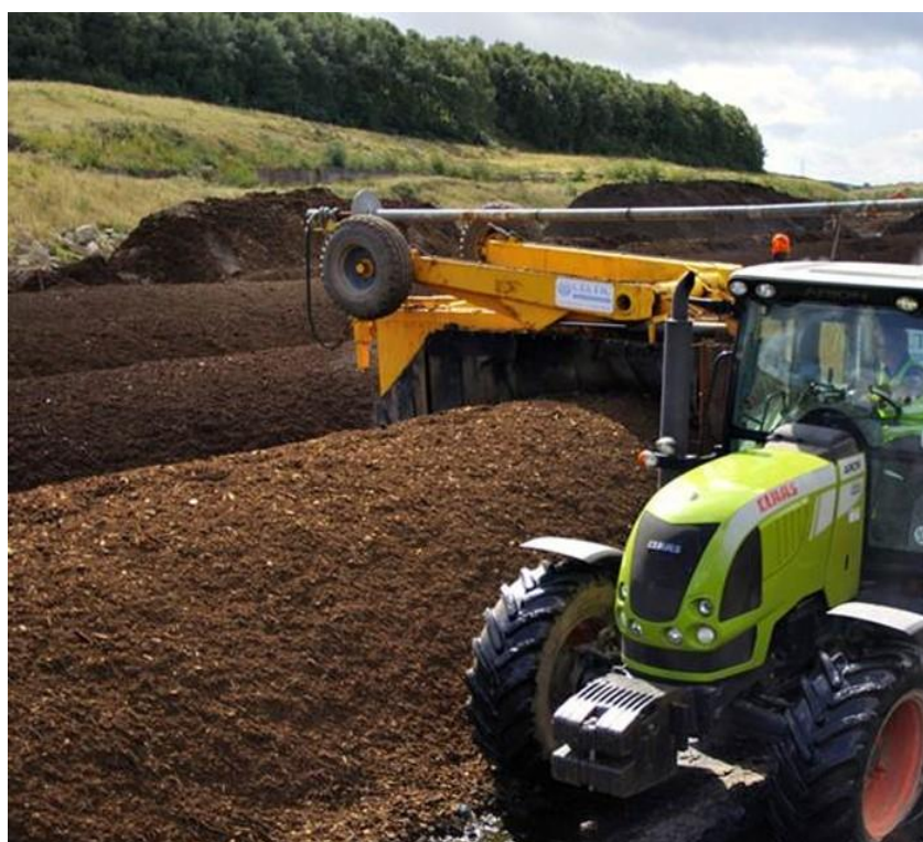
Figure 1-2 Bioremediation Process – Mechanical Turning
