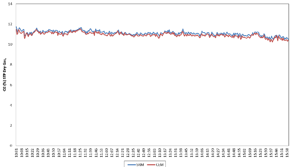
Time Series Plot of SRM and CEM O2 Readings A2 FB-001 on 09/09/2015
