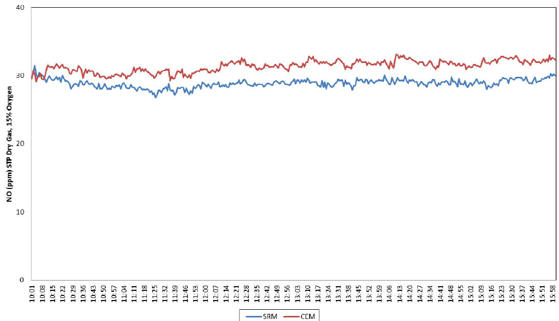
Time Series Plot of SRM and CEM NO Readings A2 FB-001 on 09/09/2015
